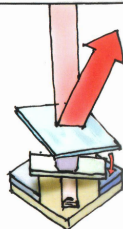
MIRROR IS "OFF" Micromirror reflects light away from the projector's main mirror.
