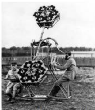
Figure 1: Acoustic array developed by Sergeant Jean Perrin (right) and used by the French Army during WWI to detect enemy aircraft.
