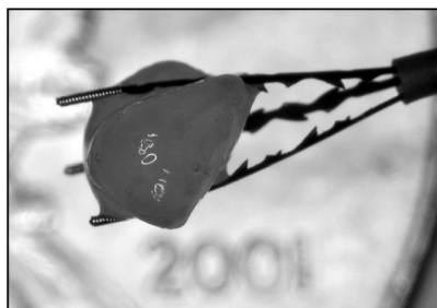
Figure 3. This grasper (cut from 0.3-mm-diameter Nitinol tubing) is designed to percutaneously retrieve embolized occlusion coils from the neurovascular system. Reaching the arterial system of the brain from the groin requires a shaft that is exceedingly small, flexible, and kink-resistant.
