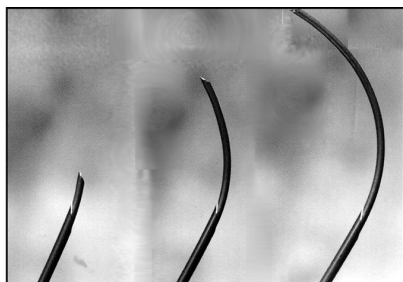
Figure 2. The SmartGuide™ is a deflectable, multipurpose 2.0-mm-diameter needle produced by Daum. It can be deflected at a 90° angle by advancing a curved Nitinol tube from stiffer, straight tubing. Such redirection applications become a commonplace use of superelasticity due to the abruptness with which the redirection can be affected.
