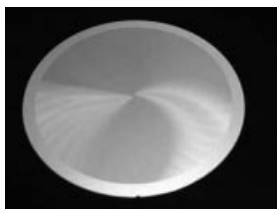
Figure 12.7 Bonded pair (200mm) with 200°C post-bonding anneal. The top silicon was thinned down to 5 μm with successive coarse and fine grinding.
