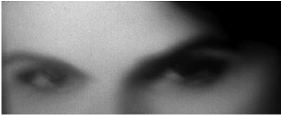
Figure 13.7 Unfocused image from 1.5 megapixel, 1.25 μm pixel pitch, 3D BIS-CIS built with nickel DBI® hybrid bonding.
