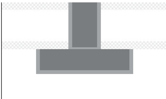
Figure 13.3 Hybrid copper/silicon nitride surface before hybrid bonding.
