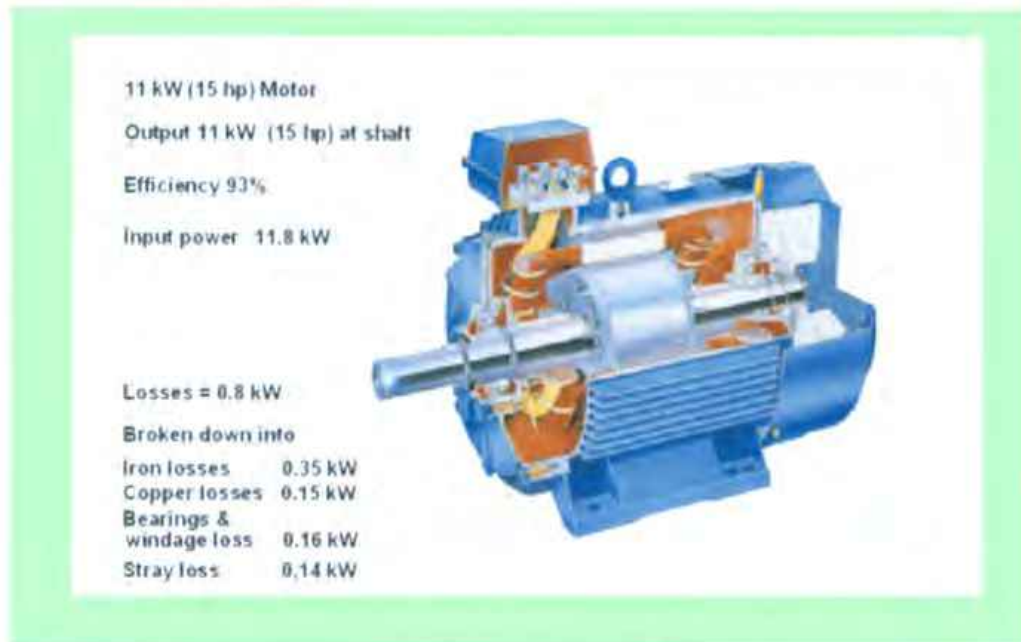
Figure A6.3: Typical motor losses
