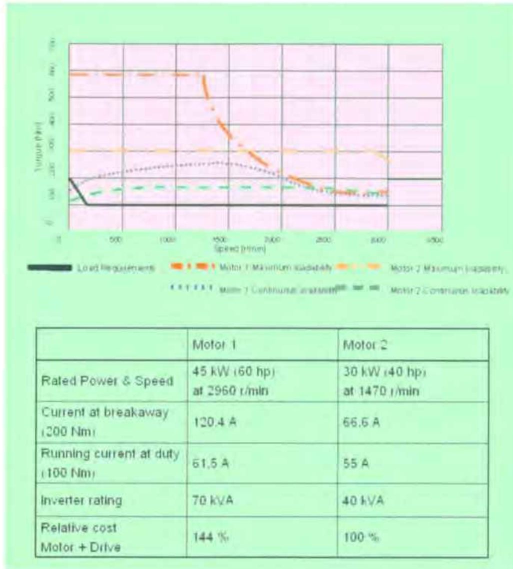
Figure 11.4: Motor load capability curves
