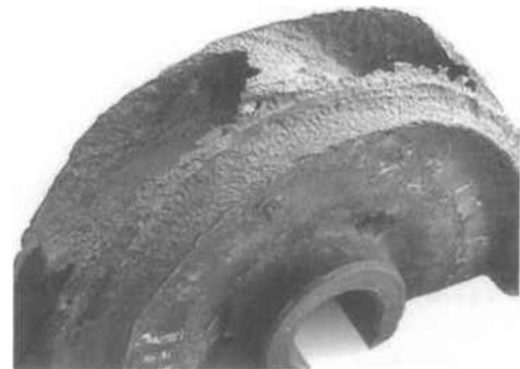
Figure 7.20 Severely damaged pump impeller
