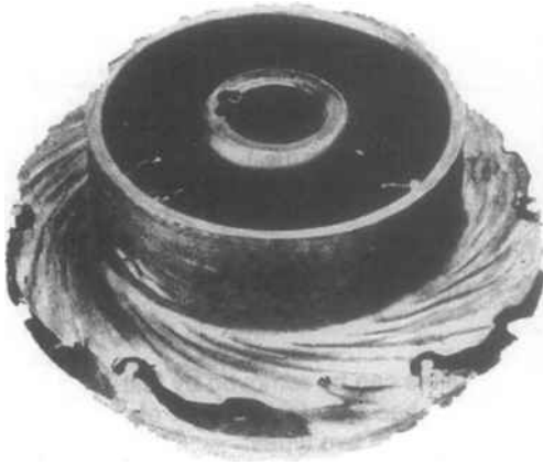
Figure 7.12 Erosion-corrosion on a 13Cr + Mo steel impeller
