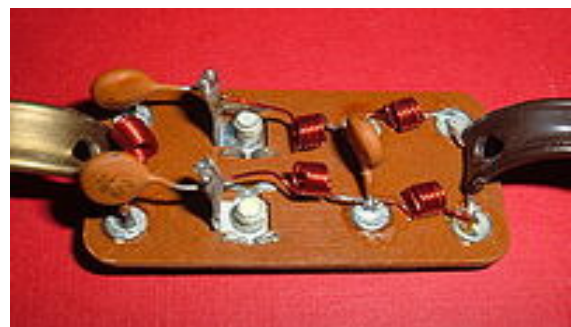
Fig.4. TV signal splitter with of a passive High-pass filter (left) and a passive low-pass filter (right). [6]
