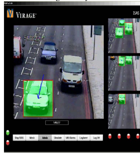
Fig 6. Automated Vehicle Location System
