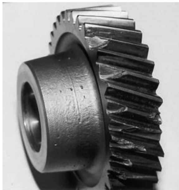
Fig. 1. General appearance of the failed helical gear.
