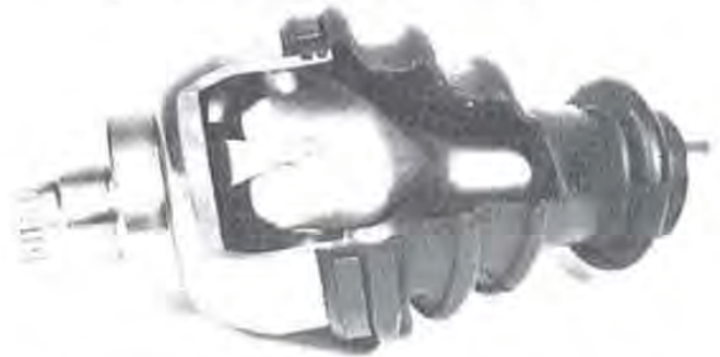
Fig. 3 — Typical assembly retention feature of fixed center tripot joint
