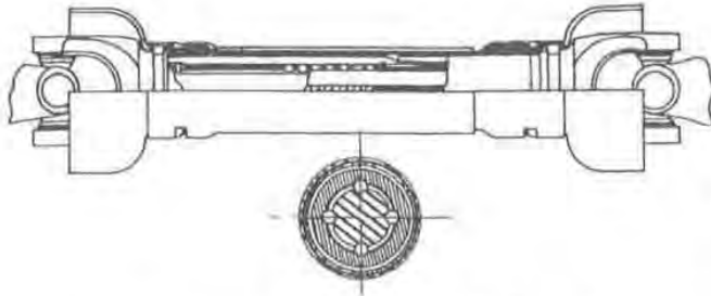
Fig. 25 — Nonrecirculating ball spline in a power take-off driveshaft
