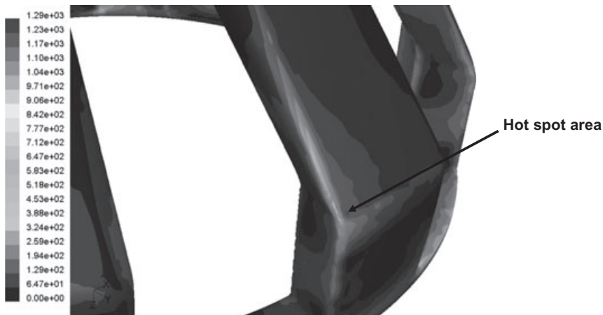
FIG. 8. Contours of wall shear stress on rotor A. A hot spot region exists on the leading edge.
