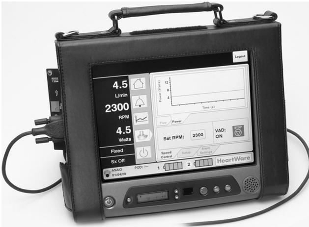
Figure 3. The monitor is a tablet PC with touch screen function. The monitor is used during system initiation, during the immediate postoperative time, and during routine checks or troubleshooting for ambulatory patients.
