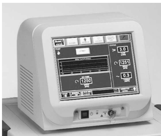
Fig 2. DuraHeart console, which enables monitoring of the system and adjustment of the pump parameters, and can store system and pump data.
