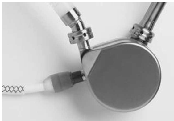
Fig 1. Pumping unit. The DuraHeart VAD has a displacement volume of 180 cm 3 and a weight of 540 g. The external dimensions are 72 mm in width and 45 mm in height.
