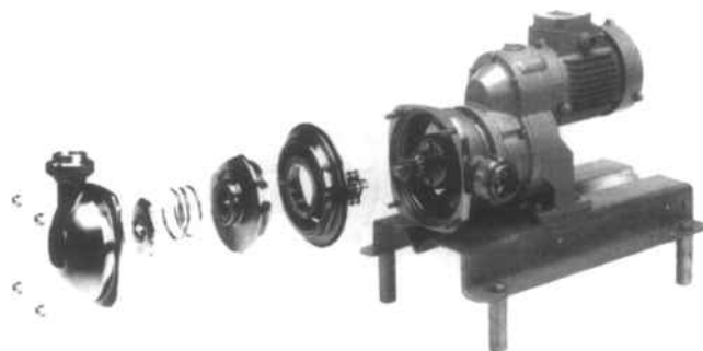
Figure 1.88 Exploded view of an eccentric drive pump
