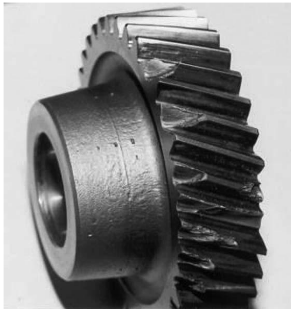
Fig. 1. General appearance of the failed helical gear.
