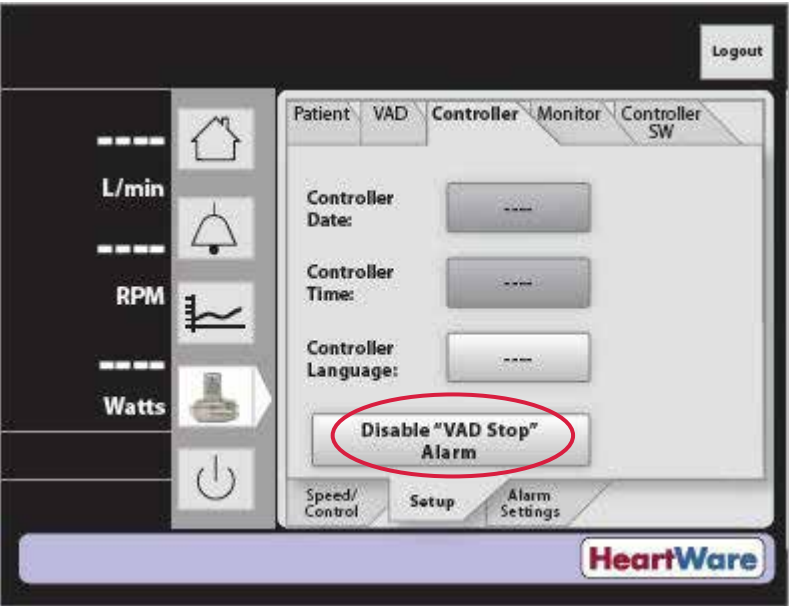
Figure 85: Disable “VAD Stop” Alarm
