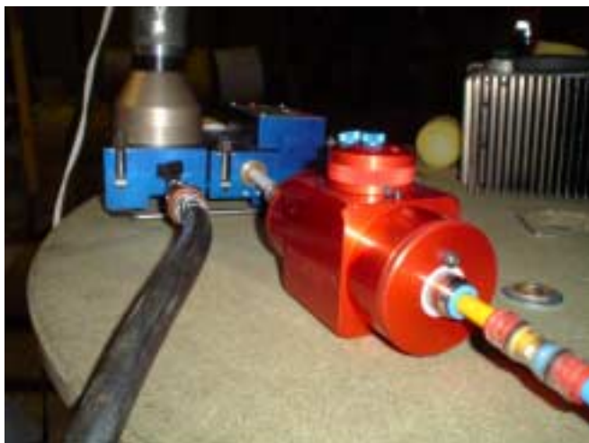
Figure 5. Cable blowing equipment (blue apparatus) and cable lubricator (red apparatus)
