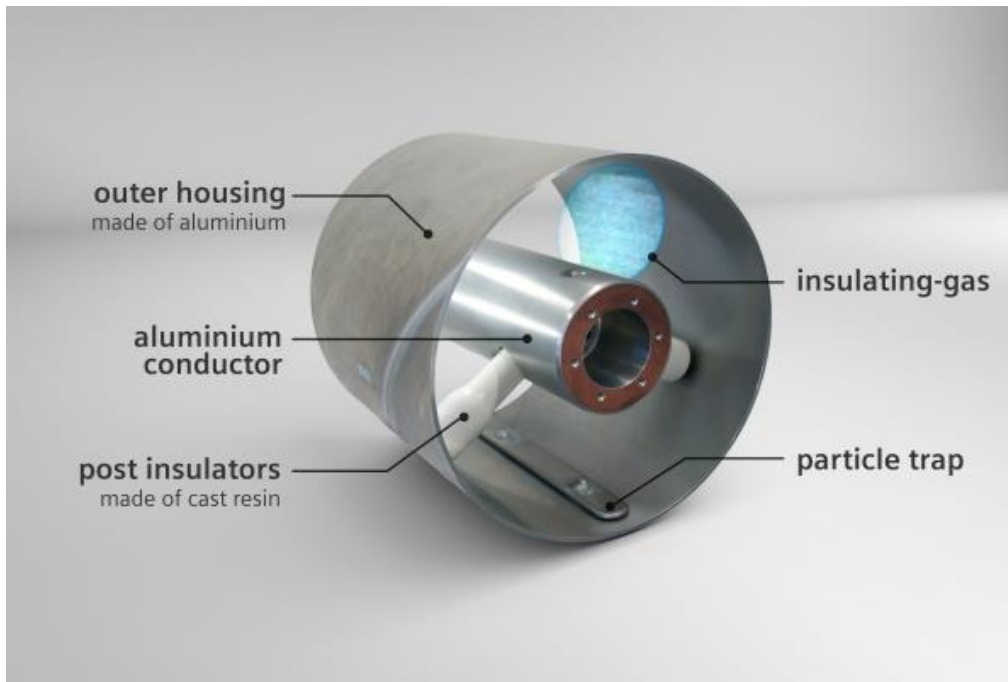
Figure 8-6: GIL Cross Section (courtesy of Siemens) [75]
