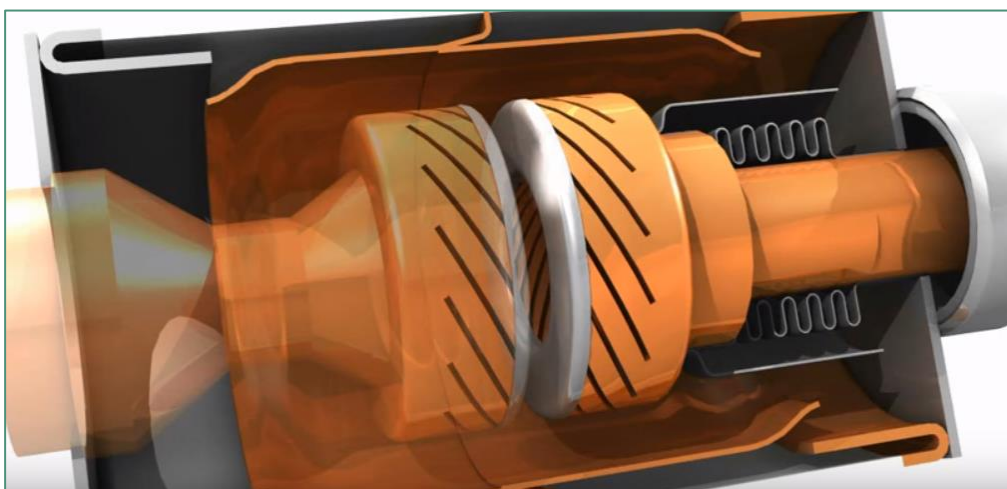
Figure 3-6: Vacuum Circuit Breaker Contact Illustration [30]
