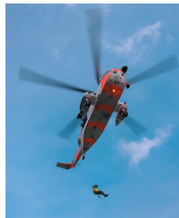
Figure 10.22 The rotational kinetic energy of a helicopter's main rotor is equal to the total work done to set it spinning. When it is spinning at a constant rate, positive work is done on the rotor by the engine and negative work is done on it by air resistance. Hence the net work being done is zero and the kinetic energy remains constant.
