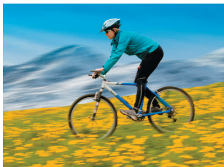
Figure 10.17 The axle of a bicycle wheel passes through the wheel's center of mass and is an axis of symmetry. Hence the rotation of the wheel is described by Eq. (10.13), provided the bicycle doesn't turn or tilt to one side (which would change the orientation of the axle).
