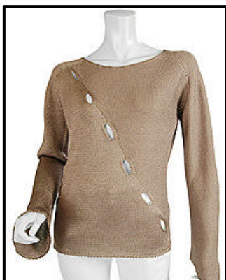
Figure 4.1. Seam free garment created on Shima Seiki WholeGarment® Machine (Shima Seiki, 2003)
