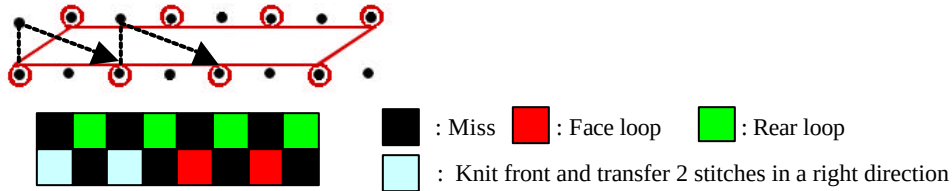
Figure 7.1.2c. Loop transference on front bed for seamless garment knitting
