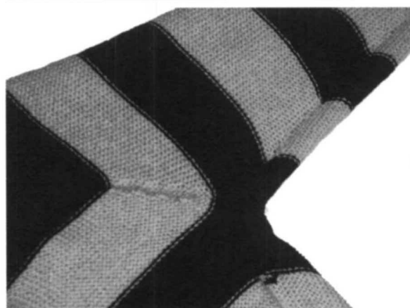
Figure 6. Seamless garment turned inside out to show the joining of the body and sleeve tubes at the underarm. This process omits uncomfortable underarm seams.
