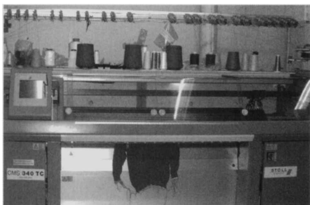
Figure 2. Seamless knitted jumper on a Stoll-knit and wear ® machine.
