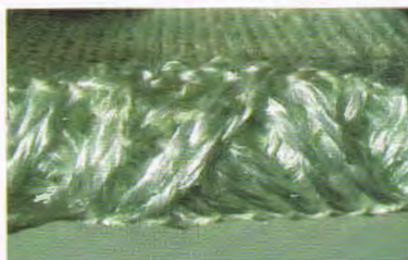
Fig. 1 Knitted spacer structure in coarse gauge, made of glass fiber yarn
