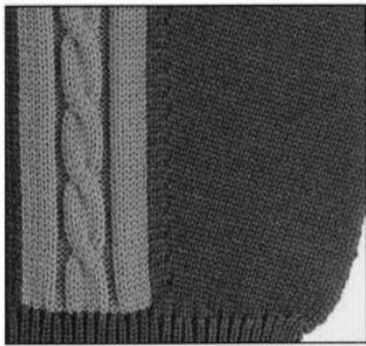
Widening with split-stitch (latch-type needle)
