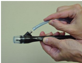
Figure 8: Connect Vacuum Tubing to Handpiece
