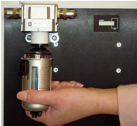
Figure 15a: Release External Air Filter
