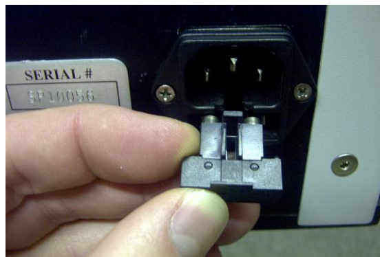
Figure 16b: Remove Fuse Box
