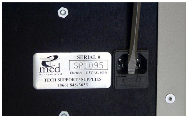
Figure 16a: Slide Out Black Fuse Box
