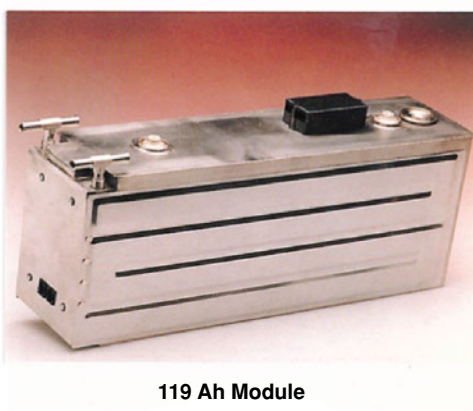
FIGURE 11 Concept and module of the all-solid advanced electric vehicle battery using a dry polymer electrolyte and a metallic lithium anode developed jointly in 1993 by 3M and Hydro Québec under U.S. Advanced Battery Consortium contracts. The goal was to produce a series of full-sized lithium polymer battery packs for extensive platform and road testing. Unfortunately, despite initial success, the project was abandoned.
