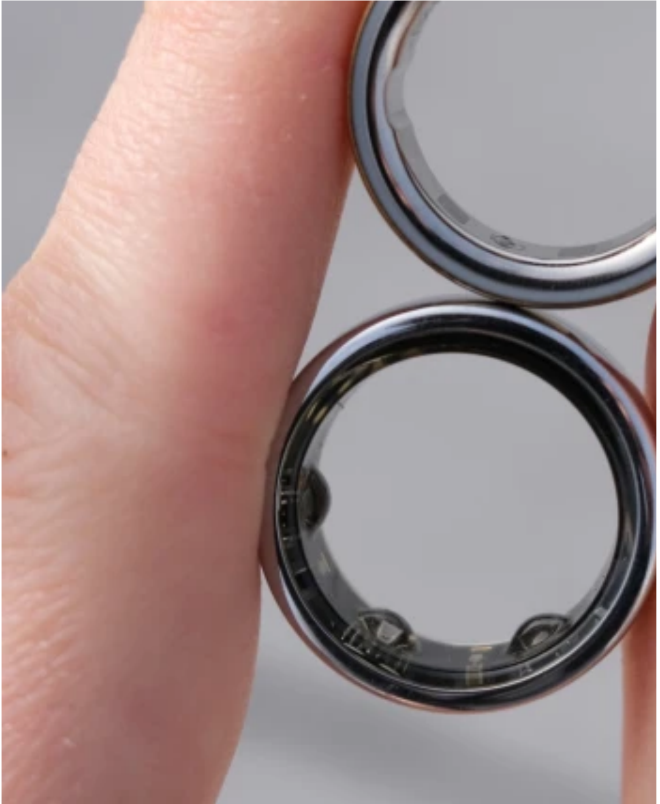
— The smooth interior of the Oura Ring 4 (top) versus the bumps on the Oura Ring Gen 3 (bottom) Courtesy Harry Rabinowitz
