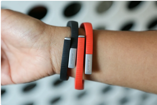
The ends of the Up24 do not clasp, but wrap around your wrist parallel to each other.
