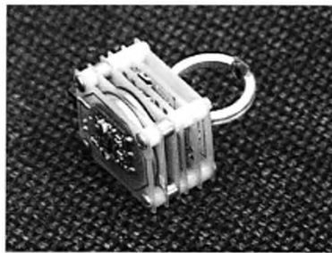
Figure 8-1 First Prototype Ring Sensor
