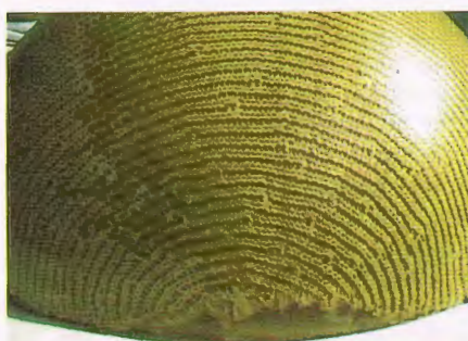
Fig. 3 Spherical shaped, knitted helmet reinforcement inlay, made of glass fiber/p-aramid blend
