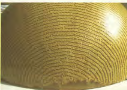
Fig. 3 Spherical shaped, knitted helmet reinforcement inlay, made of glass fiber/p-aramid blend
