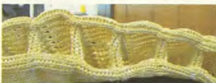
Fig. 2 Knitted web or interface structure of a glass fiber/p-aramid blend
