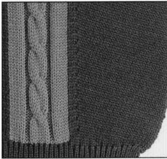
Widening with split-stitch (latch-type needle)
