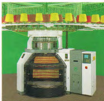
The Relanit 1.6 R is capable of knitting twelve-colour stripes
