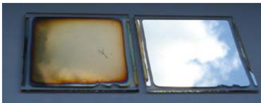
Fig. 27 Photo of already tarnished Ag/glass (left), and bright \text{Al}_2\text{O}_3 /Ag/glass (right). The samples have been aged almost four years at room atmosphere. Mirrors show Finnish cloudy summer sky taken with a digital camera without flash and the photo has not been processed in any way.
