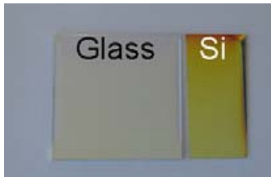
Fig. 25 Photograph of HLHLHLHLH multilayer stack deposited on glass (left) and on Si (right). The samples lie on a white paper. H is \text{Ta}_2\text{O}_5 film and L is \text{MgF}_2 .
