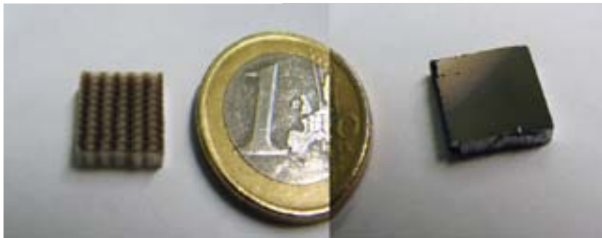
Fig. 33 Photos of un-coated (left) and Ir-coated (right) MCPs. One euro coin is just shown as a reference. 179
