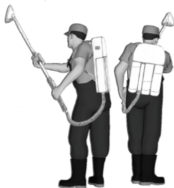
Figure 2-2: Conceptual sketch of sign cleaning tool
