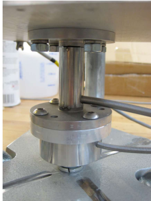
Figure 3-9: Torque cell and load cell affixed between test bed and stand
