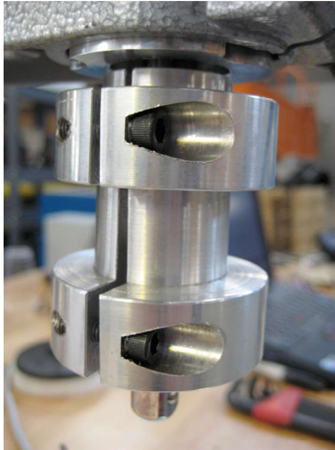
Figure 3-6: Coupling from shaft to brush
