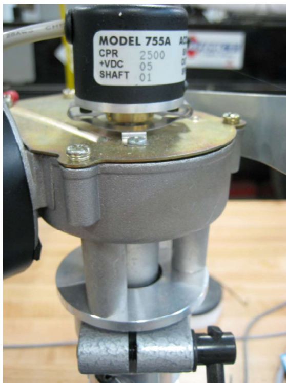
Figure 3-14: Encoder attached to back of motor
