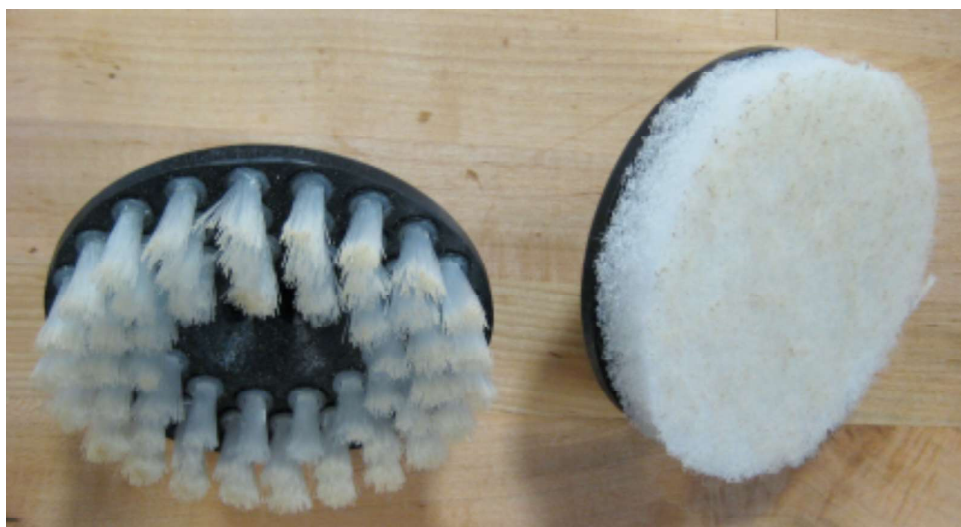
Figure 3-10: Brushes used in tests. Left: Polypropylene; Right: Scouring Pad
