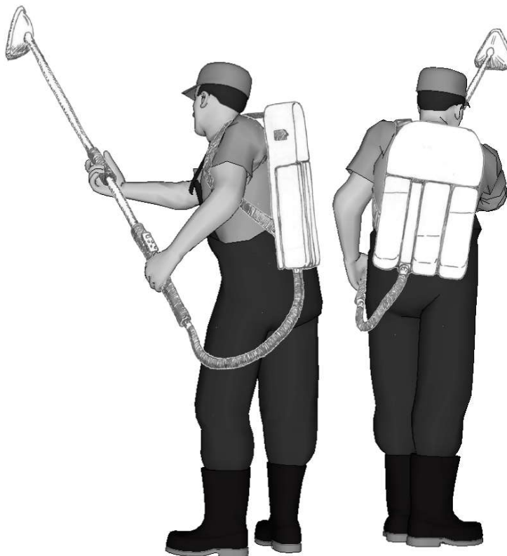
Figure 2-2: Conceptual sketch of sign cleaning tool
