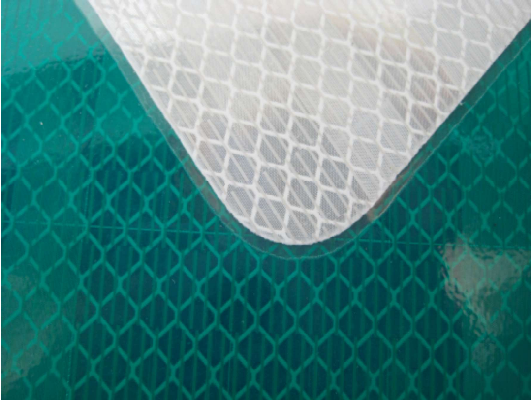
Figure 1-4: Microprismatic film, different layers of lettering and background
