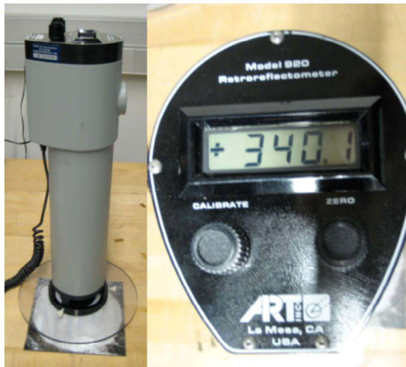
Figure 3-16: Retroreflectometer; Detail of calibration knobs and readout
