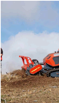
Seppi M.'s Max 50 le Is a Remote Controlled Tracked Tool Carrier
