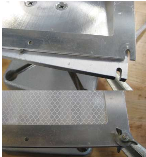
Figure 3-8: Detail of test bed showing frame attachment method
