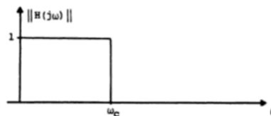
Fig. 1.23. Ideal LP filter magnitude frequency response.
