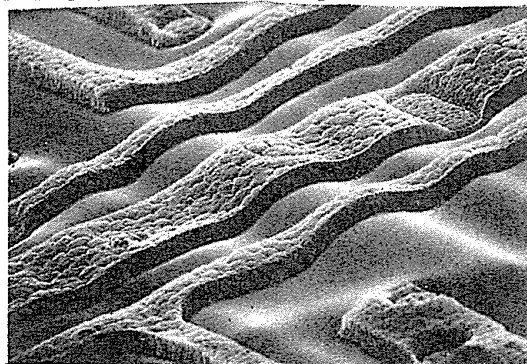
Fig. 22 Micrographs showing BPSG as the interlevel dielectric under the metal. Reprinted with permission of Semiconductor International 2 .
