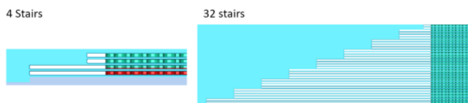
Figure 3: SiN sacrificial layer issues. Removal of SiN is required to create the ONON stack 3D structure in a 3D NAND. The left diagram displays a 20~30 nm thick SiO 2 layer bridged over a 500 nm distance. With larger staircases (see right diagram), the oxide layer spans a greater dimension and there is a danger of layer collapse.
