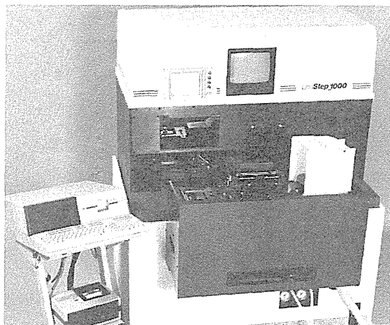
Fig. 17 1X Stepper. Courtesy of Ultratech Stepper.
