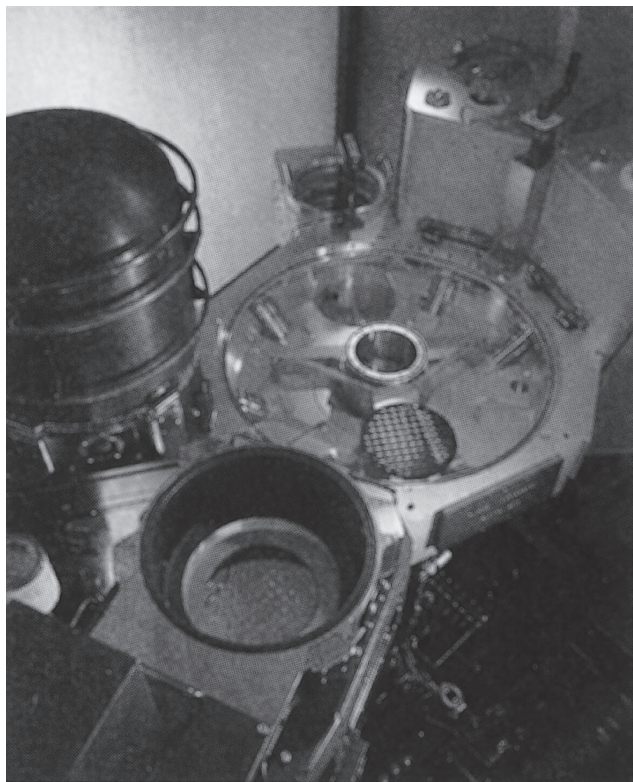
Figure 11.23 The Applied Materials high density plasma silicon etch system (photo courtesy of Applied Materials).
