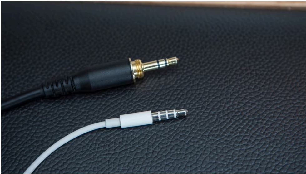
The headphone jack's metallic tip, ring and sleeve components are separated by thin insulators, coloured black in the top example and white in the lower one. Note the additional ring on the iPhone connector, which added microphone functionality to mobile headset/earphone combos. (Evan Mitsui/CBC)
