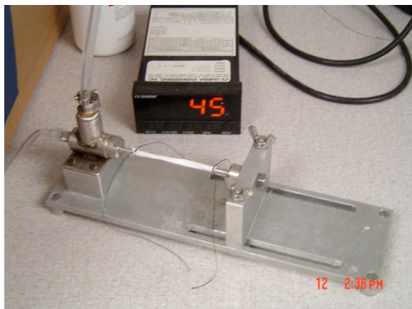
Fig. 2 – Image of the custom burst strength device. In this image, air flows from a pressure regulator into the graft. Graft pressure is measured with a pressure transducer.
