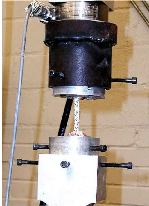
Fig. 2. BPTB complex mounted on tensile testing machine for tensile testing.
