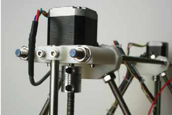
Figure 10-8. Aluminum helical coupler on a RepRap z-axis
