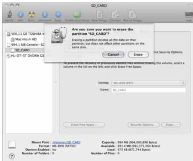
Figure 10-22. Formatting an SD card on a Mac
