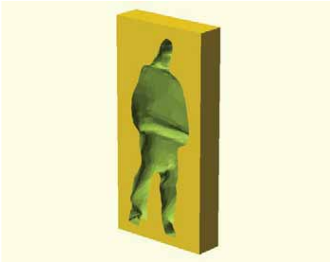
Figure 7-6. The negative shape of an imported STL
