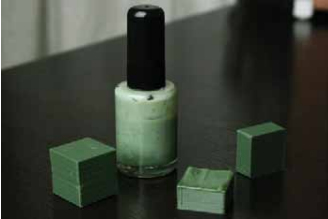
Figure A-15. Finished ABS cement
