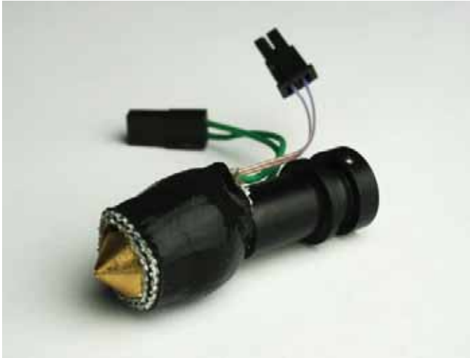
Figure 3-14. MakerGear hotend with 0.35mm brass nozzle
