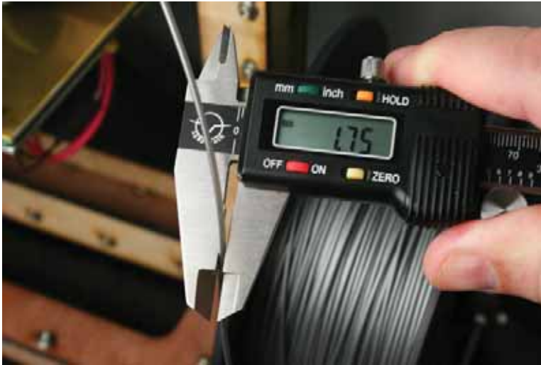
Figure 3-15. Measuring filament diameter
