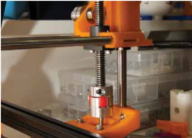
Figure 10-9. MendelMax z-axis with spider coupler (courtesy Tommy Cheng, 2012)
