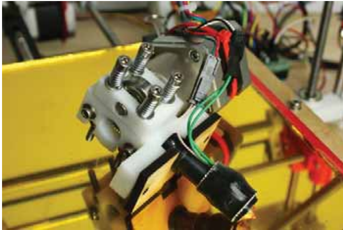
Figure 10-27. MakerGear stepper extruder
