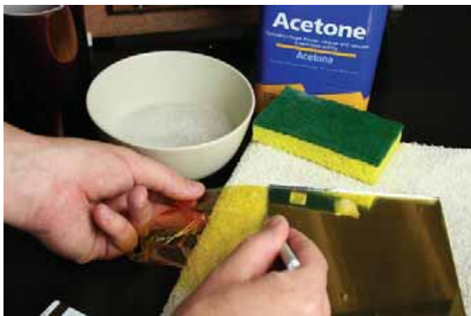
Figure A-7. Trimming polymide tape with a hobby knife
