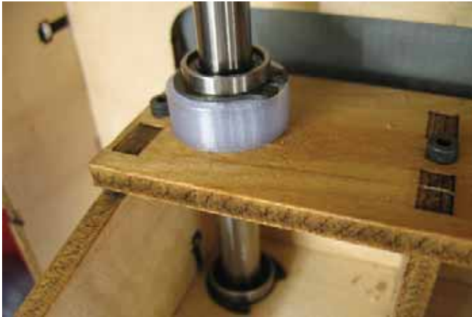
Figure 10-7. Linear bearing installed on a Thing-O-Matic z-axis (courtesy Tony Buser, 2012)
