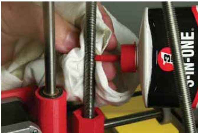
Figure A-2. Applying machine oil to a Prusa Mendel leadscrew
