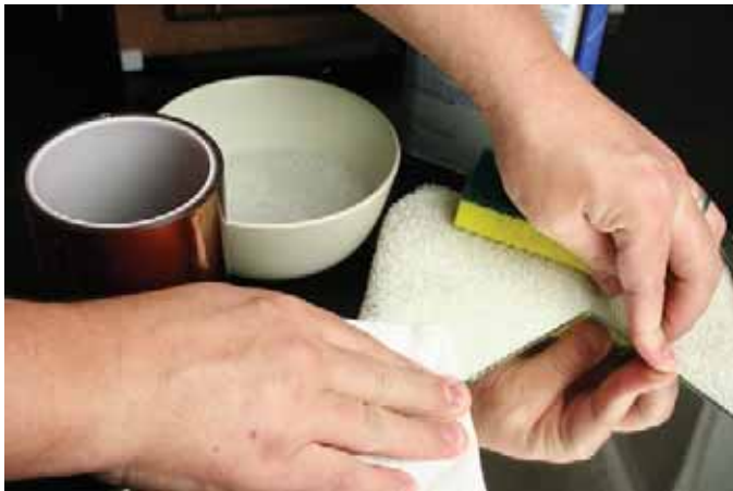
Figure A-3. Cleaning the printbed surface
