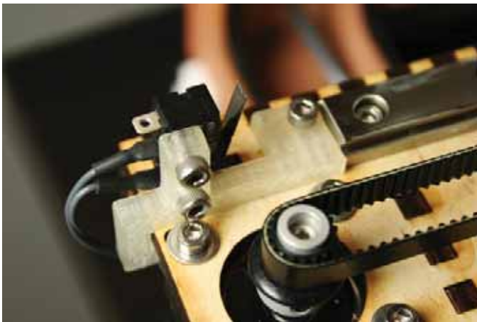
Figure 10-10. Y-axis minimum endstop on a MakerGear Mosaic
