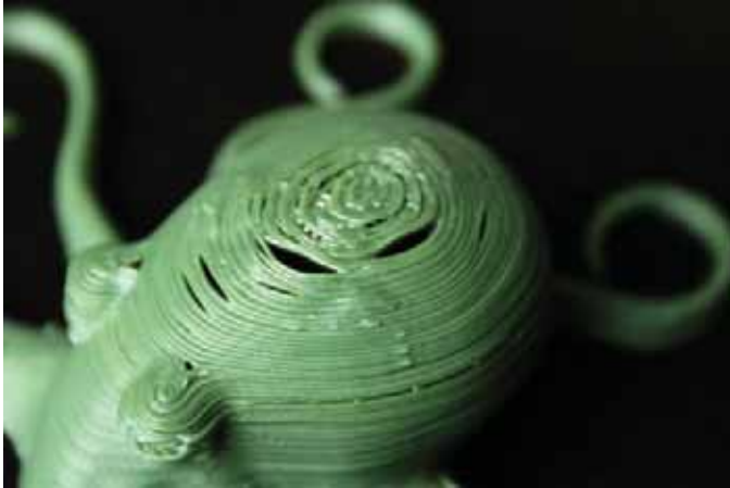
Figure A-13. Gaps in a print
