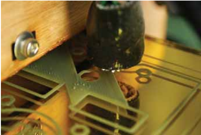
Figure A-9. First layer of a new print
