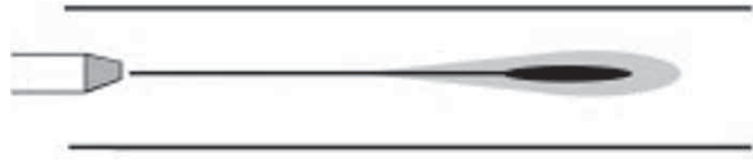
5.4 Diffusion of dye in water flowing through a tube.
