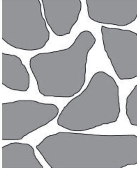
5.8 Schematic diagram of a porous solid.
