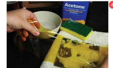
Figure A-5. Applying polyimide tape to soapy surface
