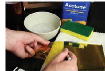
Figure A-7. Trimming polyimide tape with a hobby knife
