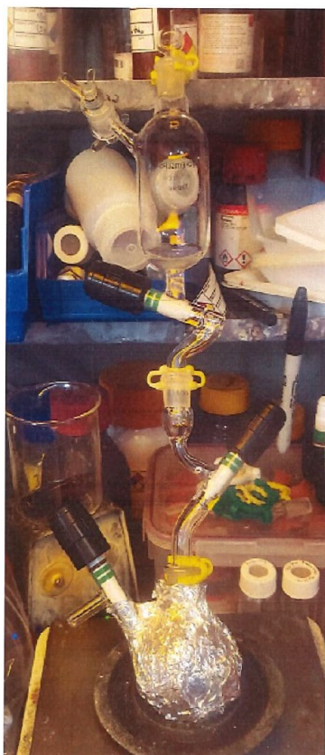
Figure 1. Air free addition setup with \text{Sn}(\text{NEt}_2)_4 in the flask and ^t\text{BuLi} in the addition funnel.
