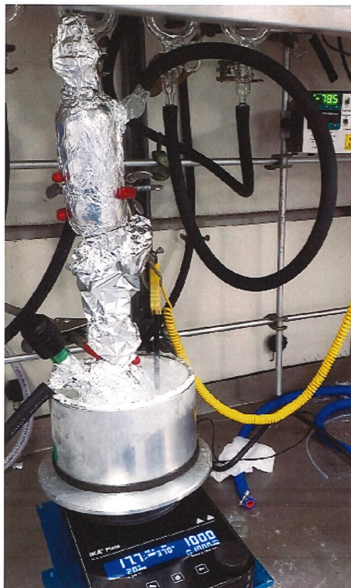
Figure 22. Air free addition setup attached to the Schlenk line with the \text{LiNMe}_2 suspension being cooled in an isopropanol liquid nitrogen bath ( -78^\circ\text{C} ).
