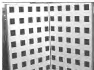
Fig. 7.1. An image of a typical calibration object. The black and white checkerboard pattern (a "Tsai grid") is designed to enable the positions of the corners of the imaged squares to be obtained to high accuracy. A total of 197 points were identified and used to calibrate the camera in the examples of this chapter.
