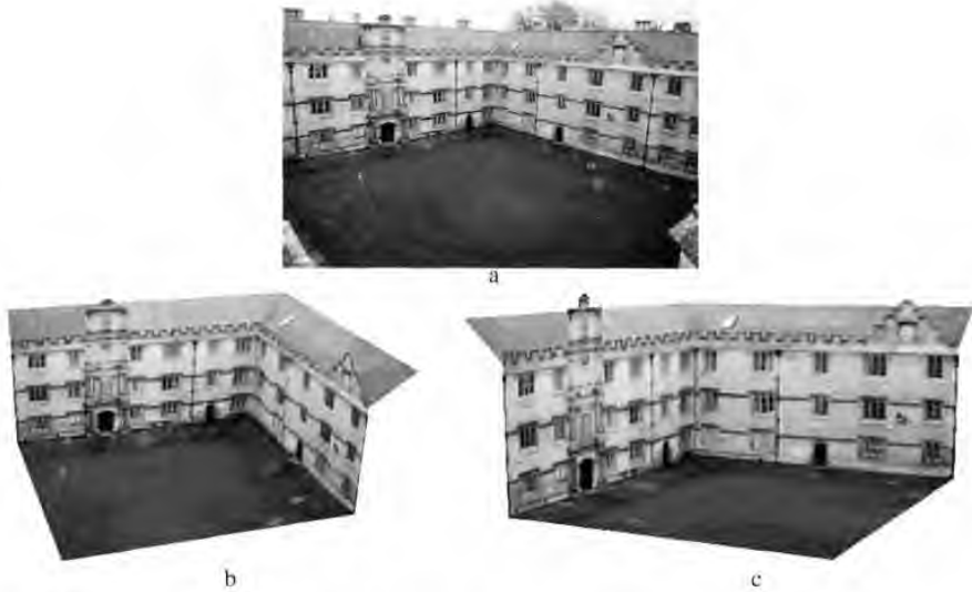
Fig. 8.26. Single view reconstruction. (a) Original image of the Fellows quad, Merton College, Oxford. (b) (c) Views of the 3D model created from the single image. The vanishing line of the roof planes is computed from the repetition of the texture pattern.
