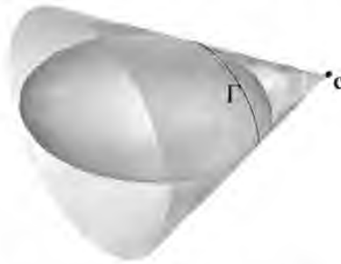
Fig. 8.4. The cone of rays for a quadric. The vertex of the cone is the camera centre. (a) The contour generator \Gamma of a quadric is a plane curve (a conic) which is the intersection of the quadric with the polar plane of the camera centre, C .
