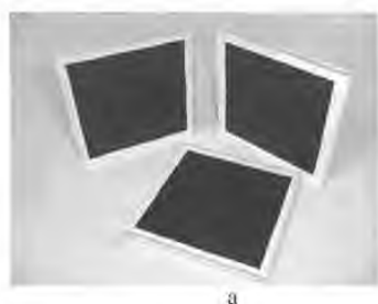
Fig. 8.12. Calibration from metric planes. (a) Three squares provide a simple calibration object. The planes need not be orthogonal. (b) The computed calibration matrix using the algorithm of example 8.18. The image size is 1024 \times 768 pixels.
