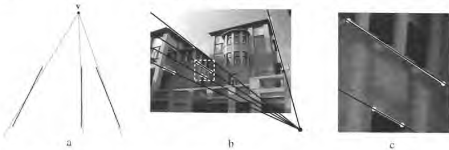
Fig. 8.15. ML estimate of a vanishing point from imaged parallel scene lines. (a) Estimating the vanishing point v involves fitting a line (shown thin here) through v to each measured line (shown thick here). The ML estimate of v is the point which minimizes the sum of squared orthogonal distances between the fitted lines and the measured lines' end points. (b) Measured line segments are shown in white, and fitted lines in black. (c) A close-up of the dashed square in (b). Note the very slight angle between the measured and fitted lines.
