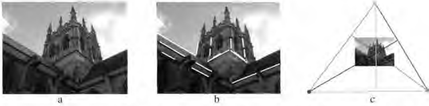
Fig. 8.22. For the case that image skew is zero and the aspect ratio unity the principal point is the orthocentre of an orthogonal triad of vanishing points. (a) Original image. (b) Three sets of parallel lines in the scene, with each set having direction orthogonal to the others. (c) The principal point is the orthocentre of the triangle with the vanishing points as vertices.
