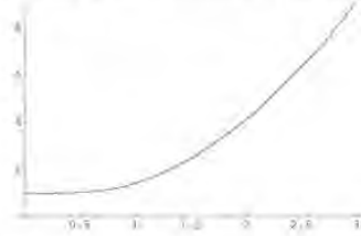
Fig. 5.5. RMS error in the position of a projected point \mathbf{x}' as a function of radial distance of \mathbf{x}' from the origin. The homography \mathbf{H} is computed from 4 evenly spaced points on a unit circle around the origin with errors in the second image only. The RMS error is proportional to the assumed error in the points used to compute \mathbf{H} , and the vertical axis is calibrated in terms of this assumed error.
